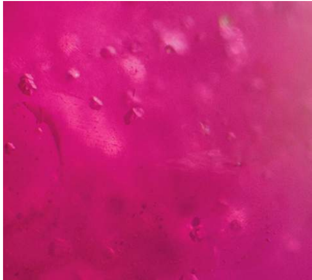
Figure 16. Negative crystals are quite common in ruby and sapphire from Tan Huong-Truc Lau, usually distributed along fractures and fissure planes. Two phases (gas and liquid) were occasionally observed in these inclusions. Photomicrograph by N. N. Khoi; magnified 45x.
