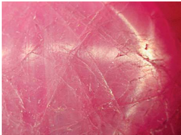
Figure 17. Asterism and growth structures are seen in this 14.45 ct pink sapphire from Truc Lau (left). Polysynthetic twinning, parallel to the positive rhombohedron r \{10\bar{1}1\} , is a common feature of ruby and sapphire from Tan Huong-Truc Lau (right). Photomicrographs by N. N. Khoi; magnified 12x.
